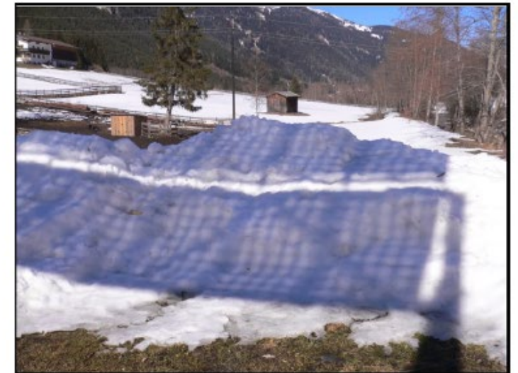
Diffuse shadows from bifacial PV modules near the ground Implementation of agrophotovoltaics thcno-economic.pdf
